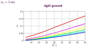
Dependences of the efficiency x of a pulse seismic source on depth  $h_i$  and angle  $\theta$  for a ground and a rigid ground
