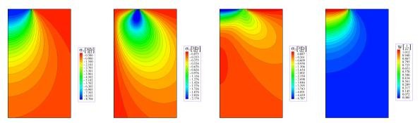
Level curves of static stresses  $\sigma_{11}$ ,  $\sigma_{12}$ ,  $\sigma_{22}$  and elastic energy W in the ground under loading platform
