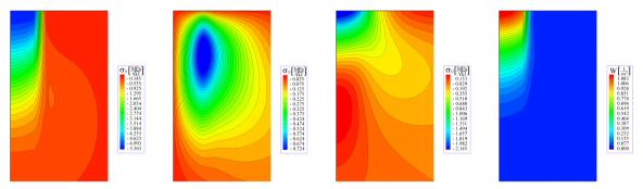
Level curves of stresses  $\sigma_{11}$ ,  $\sigma_{12}$ ,  $\sigma_{22}$  and elastic energy W in the ground under loading platform (loading time  $t_0 = 5 \text{ ms}$ )
