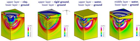
Level surfaces of tangential stress  $\sigma_{23}$  in horizontal direction (t = 18 ms)
