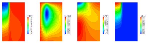
Level curves of stresses  $\sigma_{11}$ ,  $\sigma_{12}$ ,  $\sigma_{22}$  and elastic energy W in the ground under loading platform (loading time  $t_0 = 10 \text{ ms}$ )
