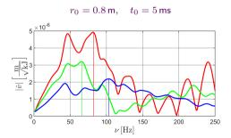
Amplitude–frequency characteristics of the velocity  $v_1$ for a ground under dynamic loading
