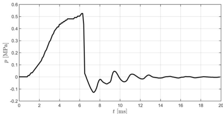
Pressure in this form was determined on the basis of experimental measurements of the acceleration of reactive mass of the electromagnet.
