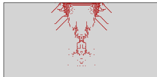
Formation and propagation of the system of interblock cracks
