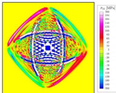
Level curves of the tangential stress depending on the thickness of interlayers
