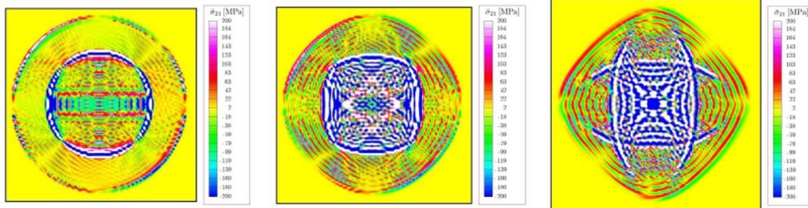
Level curves of the tangential stress depending on the thickness of interlayers
