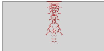
The action of  $\Pi$ -shaped smoothed pulse load on a part of the upper boundary
