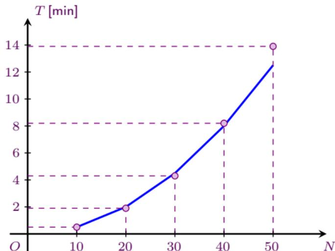
Dependence of the runtime  $T$  on the linear dimension  $N$  of a grid in blocks
