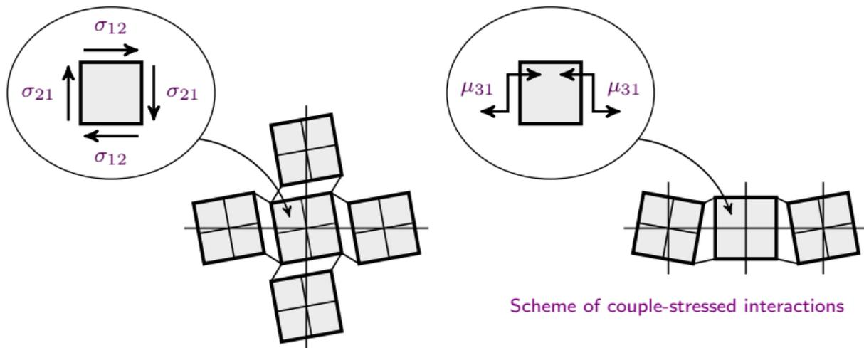
Tangential stresses caused by rotations of the blocks
